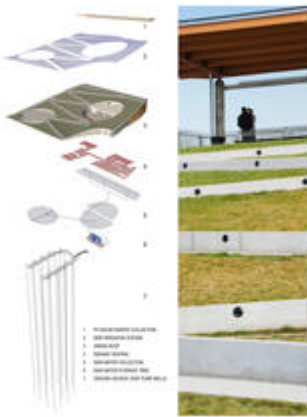
Diagram of systems and photo of Green Roof - Photo Credit: Diagram: Kiss + Cathcart, Architects © New York City, NYC Parks; Photo: © Paul Warchol
