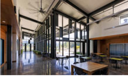
Aradiant slab and ceiling fans provide the building's heating and cooling. - Photo Credit: Stephen Miller
