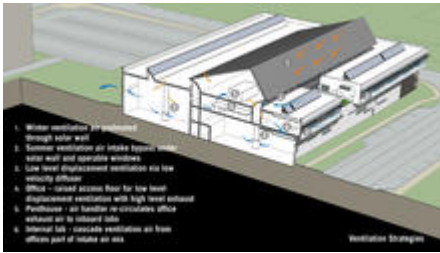
Ventilation Strategies - Photo Credit: Diamond Schmitt Architects
