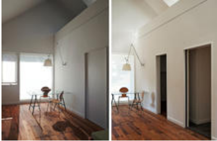
View of south window and winter light penetration (left). Conversely, the right images shows summer light penetration, as regulated by exterior shading device. - Photo Credit: Ken McCown
